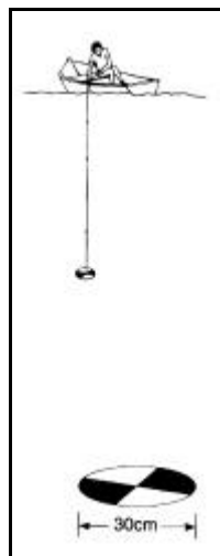
Figure 2.4 The use of a secchi disc to assess vertical water clarity. The secchi disc is lowered into the water until the black and white quarters are no longer distinguishable. The length of rope from the surveyor to the disc is then recorded (m). Source: English et al. (1997).
